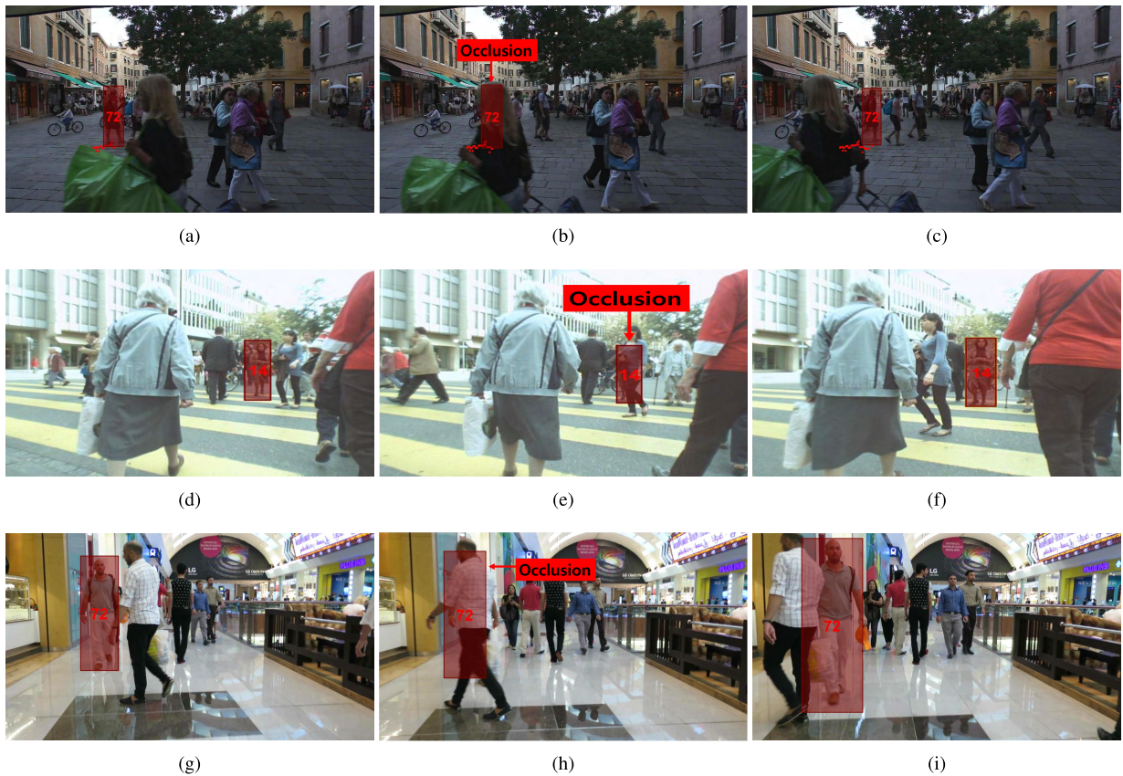
FIGURE 7. Tracking results by using our discriminative appearance learning method under occlusions. Each column shows a tracked object before/during/after the occlusion, respectively. On the sequence (MOT16-02) captured in a static camera, we also depict the trajectory of the tracked object. (a) MOT16-02 frame 452. (b) MOT16-02 frame 457. (c) MOT16-02 frame 464. (d) MOT16-05 frame 254. (e) MOT16-05 frame 259. (f) MOT16-05 frame 266. (g) MOT16-11 frame 756. (h) MOT16-11 frame 769. (i) MOT16-11 frame 782.
